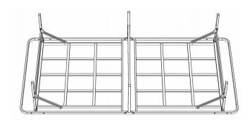
Step 3: Pull-up the support arms to hook onto the bolts .No need any tools and any components to assemble .
