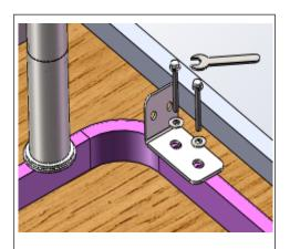
Step1:Fix the connector with 2\* 1/4\*42 screw and 2\*washer, as shown in the image.
