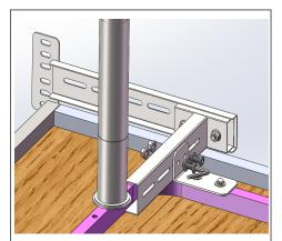
Step2:Fix the Metal Bracket-A with 2\*M8\*20 screws and 2\* nut,as shown in the image.
